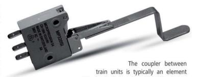
exposed to shock, dust and humidity. The mounted MP210 sealed switch detects the proper locking of the coupler. The wide temparture range of the switch of -40°C / +130°C and up to 200°C for certain models allows its use in all regions of the world and the IP67 protection keeps all dust or water off the switching circuit.
